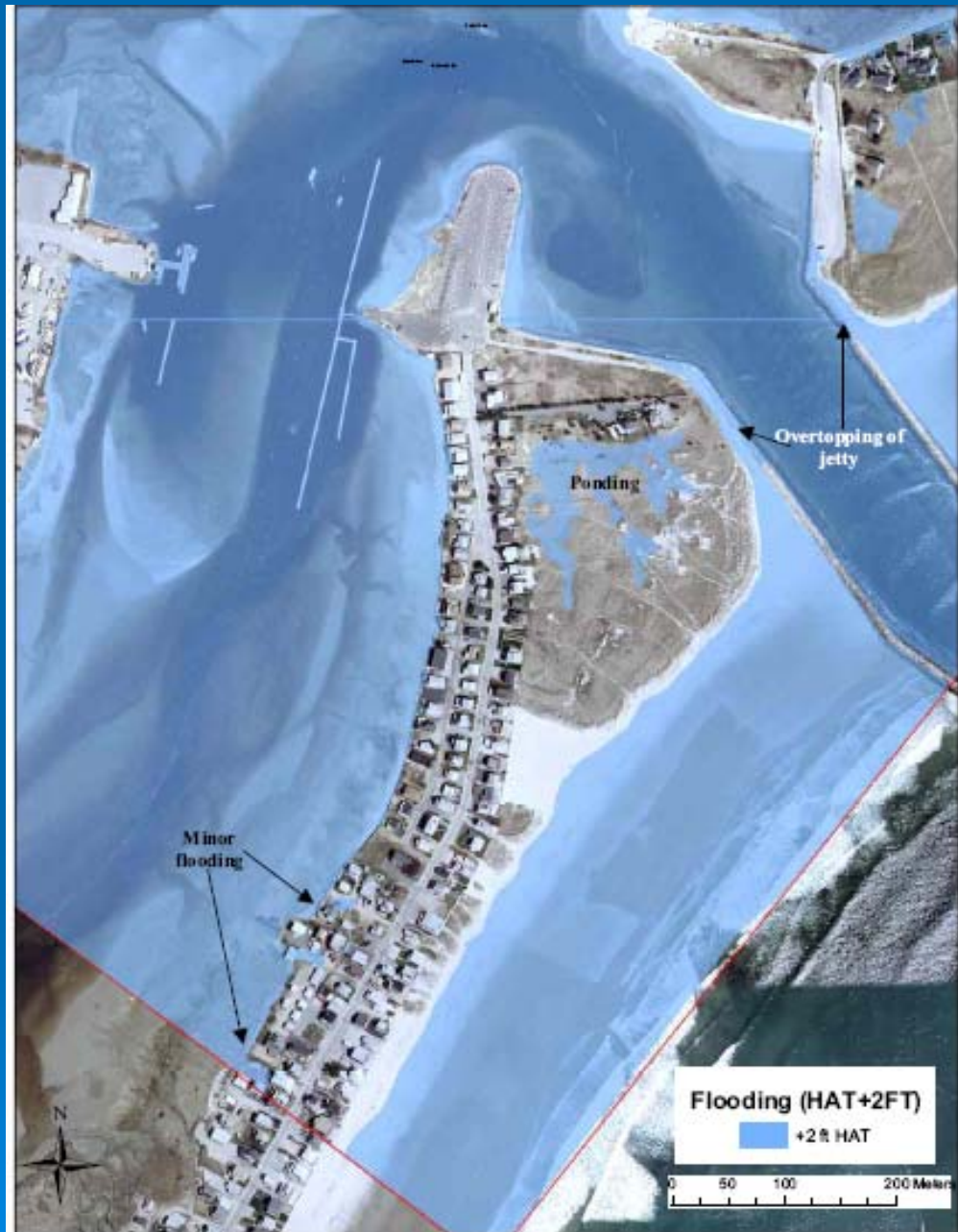
Figure 14. Simulated flooding for Wells Beach with 2 ft rise in sea level at HAT conditions. Only minor flooding is apparent on the marsh (Webbhamet River) side of the island, where several low-lying areas are flooded. Portions of the existing jetties are also overtopped.
